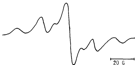
Figure 4 ESR spectrum of MAA-grafted PE film irradiated at room temperature for 30 min and recorded at -196^{\circ}\text{C} . [XT] = 0.1 wt %, grafting (%) = 56.0.
